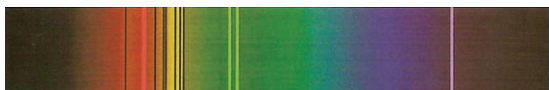
Fluorescent bulb, with energy peaks in the green and violet spectrum and missing areas in the red, orange and yellow spectrum
